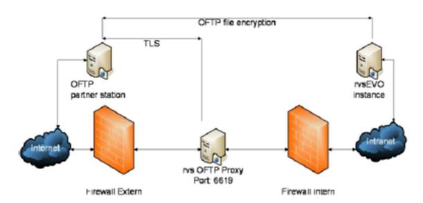
Binding of the rvs®OFTP Proxy into a rvs® based OFTP network
